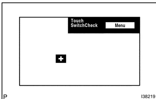
4. Touch the display anywhere in the open area to perform the check when the "Touch Switch Check" screen is displayed.
