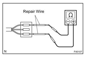
(b) Use a repair wire to check the connector if it is impossible to check continuity from the rear of the connector.
