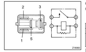
Remove the PTC heater relay from the engine room R/B. (a) (b) Measure the resistance according to the value(s) in the table below
