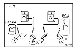
(2) Disconnect connector B and measure the resistance between the connectors.
