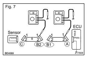
(2) Disconnect connector B and measure the resistance between terminal 1 of connector A and the body ground, and terminal 1 of connector B2 and the body ground.
