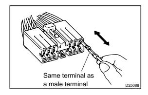
(3) Checking the contact pressure of the terminal:
