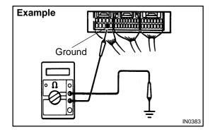
(2) Disconnect the ECU connector. Check the ground terminals (on the ECU side and wire harness side) for evidence of bending, corrosion or foreign material. Lastly check the contact pressure of the female terminals.
