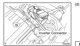
Check the connection condition of the I9 and I10 inverter connectors.
