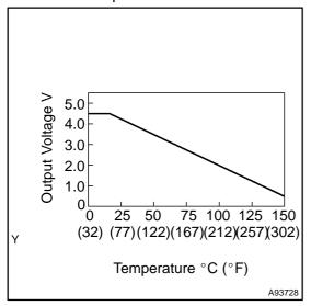
The HV control ECU uses a temperature sensor, which is built into the boost converter, to detect the temperature of the boost converter.
