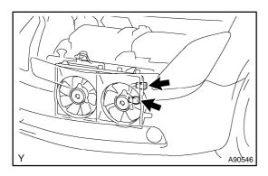
(a) Check the connection condition of the cooling fan motor connectors.
