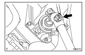
(a) Check the connection condition of the water pump connector.
