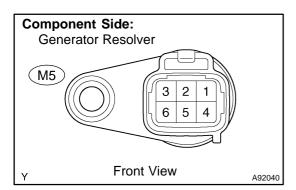
(a) Measure the resistance between the terminals of the generator resolver.
