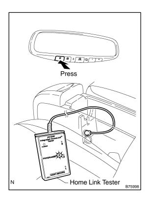
(b) Press the garage door opener switch that was registered to the tester transmitter. Check if the home link tester's green LED illuminates.
