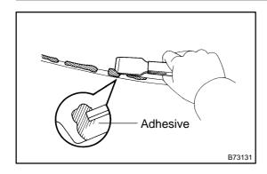
(3) Using a scraper, remove any excess or protruding adhesive.
