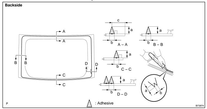
(1) Cut off the tip of the cartridge nozzle, as shown in the illustration.
