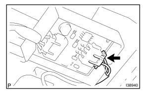
(c) Disconnect the connector and remove the amplifier microphone.
