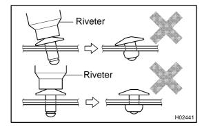
Do not tilt the riveter or remove the rivet from the material. Material that is not securely tightened may become lose.
