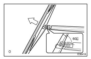
(b) Pull the rear wiper blade straight away from the rear wiper arm towards the left side of the vehicle at condition [\*1].
