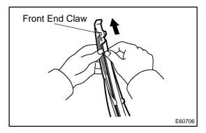
(d) Slide the rear wiper rubber through the front end claw.
