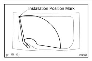
(c) Stop the rear wiper motor assy at the automatic stop position. Install the rear wiper arm assy with the nut in the position shown in the illustration.
