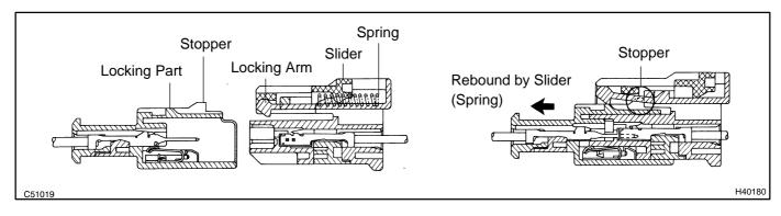
(4) Connector lock mechanism (1): Locking the connector lock button connects the connector securely.
