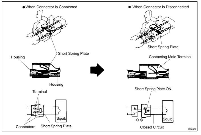
(3) Half connection prevention mechanism: If the connector is not completely connected, the connector is disconnected due to the spring operation so that no continuity exists.
