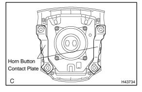
• Deformation of the horn button contact plate of the horn button assy.
