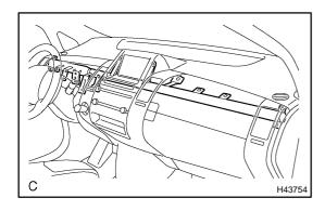
Deformation or cracks on the instrument panel or instrument panel reinforcement.
