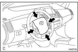
There should be no interference between the horn button assy and steering wheel assy, and the clearance should be uniform all the way around when the new horn button assy is installed on the steering wheel assy.
