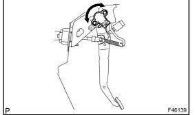
(4) Turn the power switch on (IG). Reading the stroke sensor 1 value shown on the data monitor, turn the stroke sensor slowly to the right and left to adjust it to the standard value.
