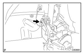
(e) Connect the front flexible hose No.1 and the speed sensor front LH to the shock absorber assy with the bolt.
