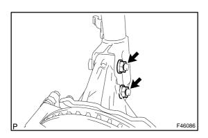
(d) Install the front shock absorber with coil spring to the steering knuckle with the 2 nuts.
