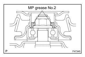
(c) Apply MP grease No.2 to the parts indicated in the illustration and install the front suspension support dust cover.
