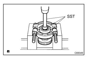
(b) Using SST and a press, remove the bearing from the counter drive gear.
