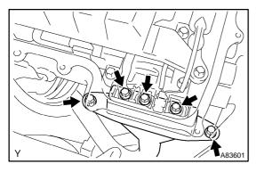
(f) Remove the 5 bolts, then disconnect the MG1 power cable.
