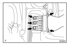
(e) Install the MG2 power cable to the MG2 power cable terminal with the 3 bolts.
