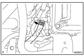
22. DISCONNECT INVERTER COOLING HOSE NO.1
