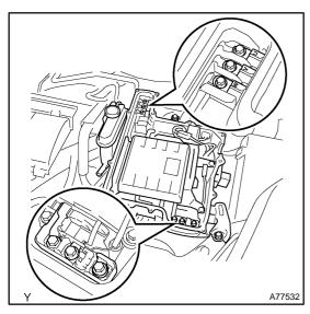
(b) Using the voltmeter, measure the voltage between the terminals of the three phase connector (U – V, V – W, U – W).
