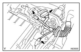
(d) Disconnect the 3 connectors shown in the illustration and the engine main wire harness.
