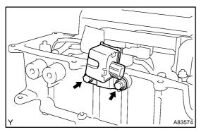
30. INSTALL CIRCUIT BREAKER SENSOR NO.1
