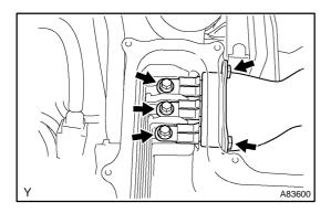
Remove the 5 bolts, then disconnect the MG2 power cable.
