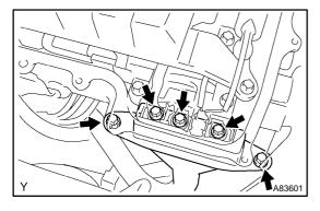
(d) Install the MG1 power cable to the MG1 power cable terminal with the 5 bolts.
