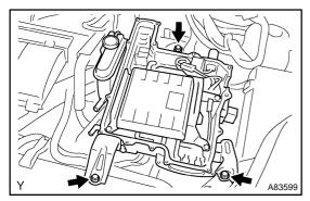
(g) Remove the 3 bolts and the with converter inverter assembly.
