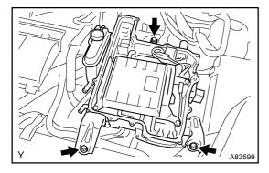
(c) Install the with converter inverter assembly with the 3 bolts.
