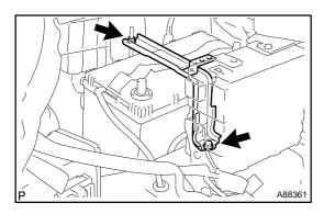
8. REMOVE BATTERY HOLD DOWN CLAMP
