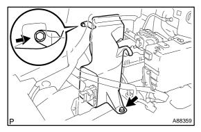
(d) Remove the bolt and screw, then remove the quarter vent duct No. 2.
