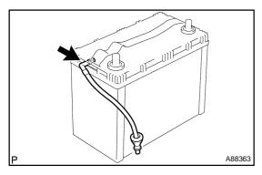
(c) Remove the battery room ventilation hose from the battery.
