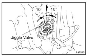
(b) Install the thermostat so the jiggle valve faces upward. HINT:
