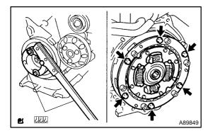
(b) Using SST, hold the crankshaft.
