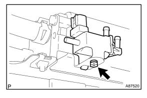
(c) Remove the bolt, then remove the charcoal canister vacuum switching valve.
