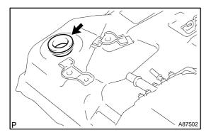
(g) Remove the gasket from the fuel tank.
