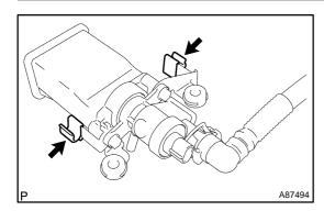
(h) Remove the 2 clamps from the trap with outlet valve canister.
