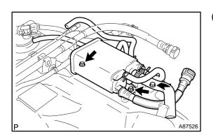
(g) Remove the bolt and 2 nuts, then remove the charcoal canister.
