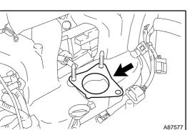
Remove the bolt and 2 nuts, then remove the throttle w/ (h) motor body.
