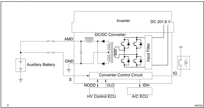
The HV control ECU uses the NODD signal line to transmit a stop command to the DC/DC converter and receive signals indicating the normal or abnormal conditions of the 12 V charging system.
