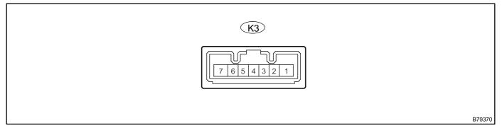
(a) Disconnect the K3 key slot connector.
