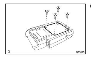
(c) Remove the 4 screws and cover using a screwdriver, as shown in the illustration.
