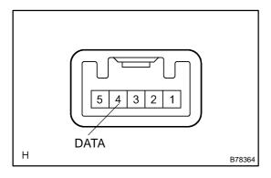
(a) Reconnect the D4 receiver connector and Measure the voltage between the terminal and body ground.
