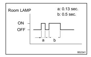
(c) Check that the system has switched to self-diagnostic mode by checking the flashes of the room lamp (dome lamp or key slot light) or buzzer outputs. Compare the flash patterns of the room lamp and output patterns of the buzzer to the timing chart on the left.
