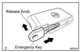
(e) Push and hold the release knob in the direction indicated by the arrow in the illustration. Insert the emergency key into the key.
