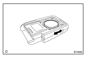
(d) Remove the transmitter's battery from the key, as shown in the illustration.
