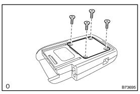
(c) Remove the 4 screws and cover using a screwdriver, as shown in the illustration.
