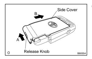
(d) Push and hold the release knob in the direction indicated by the arrow labeled A in the illustration. Push in the slide cover in the direction indicated by the arrow labeled B in the illustration and install the slide cover.
