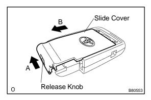
(b) Push and hold the release knob in the direction indicated by the arrow labeled A in the illustration. Push out the slide cover in the direction indicated by the arrow labeled B in the illustration and remove the slide cover.
