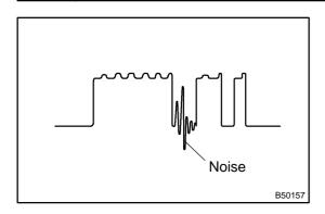
(a) Using an oscilloscope or the hand-held tester, check that the waveform between the terminals of the K3 key slot and T5 ECU connector. The waveform should be similar to the illustration on the left.
