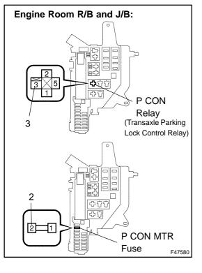
(a) Measure the resistance according to the value(s) in the table below. Standard:
