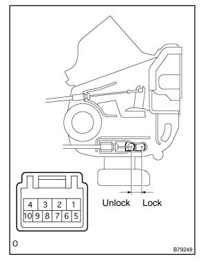
(a) Measure the resistance of the position switch. **Standard:**
