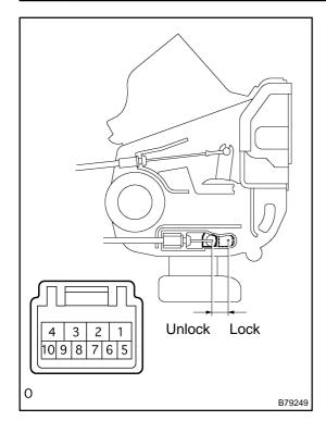
(a) Apply battery voltage to the door lock and check operation of the door lock motor.
