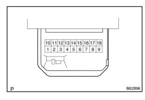
(b) Measure the resistance between the terminals of the connector when the switch is operated.
