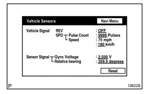
4. Check all the signals and sensors when vehicle signal information is displayed.
