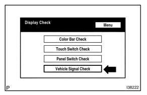
3. Select "Vehicle Signal Check" from the "Display Check" screen.
