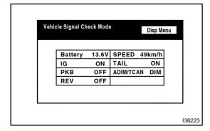
4. When the "Vehicle Signal Check Mode" screen is displayed, check all the vehicle signal conditions.
