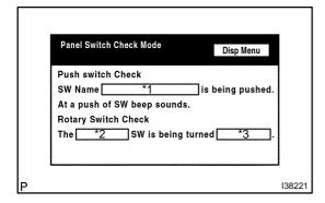
4. Operate each switch and check that the switch name and condition is correctly displayed.
