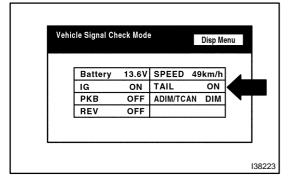
(b) Turn the light control switch TAIL or ON and OFF. **Standard:**
