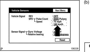
While driving, compare the "SPD" indicator to the reading on the speedometer. Check if these readings are almost the same.
