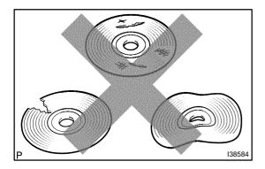
(a) Check that the map disc is not deformed or cracked.
