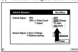
(b) While driving, compare the "SPEED" indicator to the reading on the speedometer. Check if these readings are almost the same.
