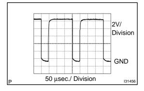
(d) Measure the waveform between terminal BLW (A8–2) of A/C amplifier and body ground.
