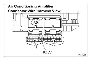
(a) Measure the voltage according to the value(s) in the table below.
