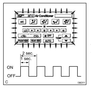
(c) The indicator check is automatically performed when activating panel diagnosis. Check that all indicators and setting displays come on and go off 4 times at 1 second intervals.
