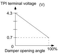
This sensor detects the position of the air inlet control servomotor and sends the appropriate signals to the A/C amplifier. The position sensor is built in the air inlet control servomotor. The position sensor's resistance changes as the air inlet control
