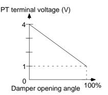
This sensor detects the position of the air mix control servomotor (air mix damper) and sends the appropriate signals to the A/C amplifier. The position sensor is built in the air mix control servomotor. The position sensor resistance changes as the air mix control servomotor arm moves.
