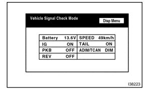
4. When the "Vehicle Signal Check Mode" screen is displayed, check all the vehicle signal conditions.
