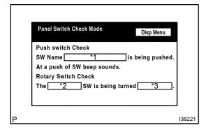
4. Operate each switch and check that the switch name and condition are correctly displayed.
