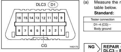
a) Measure the resistance according to the value(s) in the table below.
