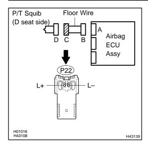
(a) Measure the resistance according to the value(s) in the table below.
